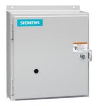
Electrically held lighting contactor, (convertible to mech. held), Amp rating 30A (tungsten 20A), 0 N.C. / 10 N.O. poles, 24V 60Hz / 20V 50Hz coil, Noncombination type, Encl NEMA type 4X 304 S-Steel, Water/dust tight noncorrosive
