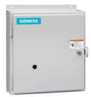
Electrically held lighting contactor, (convertible to mech. held), Amp rating 30A (tungsten 20A), 0 N.C. / 9 N.O. poles, 230-240V 60Hz/220V 50Hz coil, Noncombination type, Encl NEMA type 4X 304 S-Steel, Water/dust tight noncorrosive
