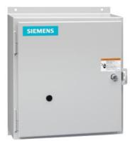
Electrically held lighting contactor, (convertible to mech. held), Amp rating 30A (tungsten 20A), 0 N.C. / 5 N.O. poles, 575-600V 60Hz/550V 50Hz coil, Noncombination type, Encl NEMA type 4X 304 S-Steel, Water/dust tight noncorrosive
