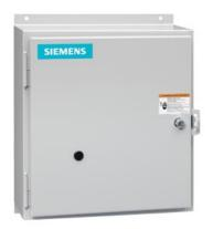
Electrically held lighting contactor, (convertible to mech. held), Amp rating 30A (tungsten 20A), 8 N.C. / 4 N.O. poles, 277V 60Hz / 240V 50Hz coil, Noncombination type, Enclosure NEMA type 12, Dust/drip proof for indoors
