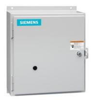
Electrically held lighting contactor, (convertible to mech. held), Amp rating 30A (tungsten 20A), 8 N.C. / 2 N.O. poles, 24V 60Hz / 20V 50Hz coil, Non-combination type, Enclosure NEMA type 12, Dust/drip proof for indoors
