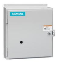
Electrically held lighting contactor, (convertible to mech. held), Amp rating 30A (tungsten 20A), 4 N.C. / 2 N.O. poles, 230-240V 60Hz/220V 50Hz coil, Noncombination type, Enclosure NEMA type 12, Dust/drip proof for indoors
