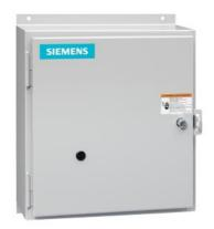
Electrically held lighting contactor, (convertible to mech. held), Amp rating 30A (tungsten 20A), 3 N.C. / 2 N.O. poles, 277V 60Hz / 240V 50Hz coil, Noncombination type, Enclosure NEMA type 12, Dust/drip proof for indoors
