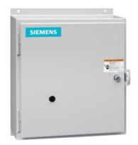
Electrically held lighting contactor, (convertible to mech. held), Amp rating 30A (tungsten 20A), 3 N.C. / 0 N.O. poles, 24V 60Hz / 20V 50Hz coil, Non-combination type, Enclosure NEMA type 12, Dust/drip proof for indoors
