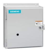
Electrically held lighting contactor, (convertible to mech. held), Amp rating 30A (tungsten 20A), 2 N.C. / 10 N.O. poles, 24V 60Hz / 20V 50Hz coil, Noncombination type, Enclosure NEMA type 12, Dust/drip proof for indoors
