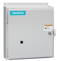
Electrically held lighting contactor, (convertible to mech. held), Amp rating 30A (tungsten 20A), 2 N.C. / 9 N.O. poles, 230-240V 60Hz/220V 50Hz coil, Noncombination type, Enclosure NEMA type 12, Dust/drip proof for indoors
