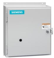
Electrically held lighting contactor, (convertible to mech. held), Amp rating 30A (tungsten 20A), 2 N.C. / 1 N.O. poles, 200-208V 60Hz coil, Non-combination type, Enclosure NEMA type 12, Dust/drip proof for indoors
