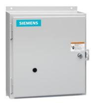
Electrically held lighting contactor, (convertible to mech. held), Amp rating 30A (tungsten 20A), 1 N.C. / 10 N.O. poles, 347V 60Hz coil, Non-combination type, Enclosure NEMA type 12, Dust/drip proof for indoors
