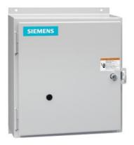
Electrically held lighting contactor, (convertible to mech. held), Amp rating 30A (tungsten 20A), 1 N.C. / 6 N.O. poles, 115-120V 60Hz/110V 50Hz coil, Noncombination type, Enclosure NEMA type 12, Dust/drip proof for indoors
