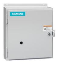
Electrically held lighting contactor, (convertible to mech. held), Amp rating 30A (tungsten 20A), 1 N.C. / 5 N.O. poles, 24V 60Hz / 20V 50Hz coil, Non-combination type, Enclosure NEMA type 12, Dust/drip proof for indoors
