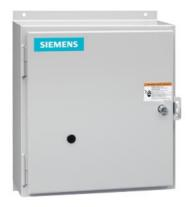
Electrically held lighting contactor, (convertible to mech. held), Amp rating 30A (tungsten 20A), 1 N.C. / 3 N.O. poles, 460-480V 60Hz/440V 50Hz coil, Noncombination type, Enclosure NEMA type 12, Dust/drip proof for indoors
