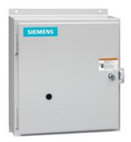
Electrically held lighting contactor, (convertible to mech. held), Amp rating 30A (tungsten 20A), 0 N.C. / 12 N.O. poles, 115-120V 60Hz/110V 50Hz coil, Noncombination type, Enclosure NEMA type 12, Dust/drip proof for indoors
