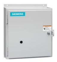
Electrically held lighting contactor, (convertible to mech. held), Amp rating 30A (tungsten 20A), 0 N.C. / 9 N.O. poles, 24V 60Hz / 20V 50Hz coil, Non-combination type, Enclosure NEMA type 12, Dust/drip proof for indoors
