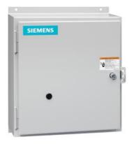
Electrically held lighting contactor, (convertible to mech. held), Amp rating 30A (tungsten 20A), 0 N.C. / 8 N.O. poles, 115-120V 60Hz/110V 50Hz coil, Noncombination type, Enclosure NEMA type 12, Dust/drip proof for indoors
