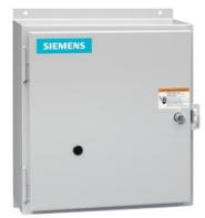
Electrically held lighting contactor, (convertible to mech. held), Amp rating 30A (tungsten 20A), 0 N.C. / 6 N.O. poles, 347V 60Hz coil, Non-combination type, Enclosure NEMA type 12, Dust/drip proof for indoors
