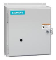
Electrically held lighting contactor, (convertible to mech. held), Amp rating 30A (tungsten 20A), 0 N.C. / 6 N.O. poles, 277V 60Hz / 240V 50Hz coil, Noncombination type, Enclosure NEMA type 12, Dust/drip proof for indoors
