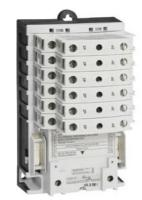
Electrically held lighting contactor, (convertible to mech. held), Amp rating 30A (tungsten 20A), 8 N.C. / 1 N.O. poles, 460-480V 60Hz/440V 50Hz coil, Noncombination type, Enclosure NEMA type (open), No enclosure
