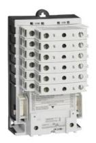
Electrically held lighting contactor, (convertible to mech. held), Amp rating 30A (tungsten 20A), 6 N.C. / 0 N.O. poles, 347V 60Hz coil, Non-combination type, Enclosure NEMA type (open), No enclosure
