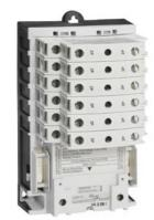
Electrically held lighting contactor, (convertible to mech. held), Amp rating 30A (tungsten 20A), 5 N.C. / 6 N.O. poles, 24V 60Hz / 20V 50Hz coil, Non-combination type, Enclosure NEMA type (open), No enclosure
