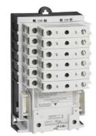
Electrically held lighting contactor, (convertible to mech. held), Amp rating 30A (tungsten 20A), 5 N.C. / 1 N.O. poles, 460-480V 60Hz/440V 50Hz coil, Non-combination type, Enclosure NEMA type (open), No enclosure
