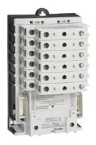
Electrically held lighting contactor, (convertible to mech. held), Amp rating 30A (tungsten 20A), 5 N.C. / 1 N.O. poles, 200-208V 60Hz coil, Non-combination type, Enclosure NEMA type (open), No enclosure
