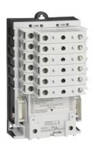
Electrically held lighting contactor, (convertible to mech. held), Amp rating 30A (tungsten 20A), 3 N.C. / 3 N.O. poles, 575-600V 60Hz/550V 50Hz coil, Noncombination type, Enclosure NEMA type (open), No enclosure
