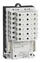
Electrically held lighting contactor, (convertible to mech. held), Amp rating 30A (tungsten 20A), 3 N.C. / 0 N.O. poles, 115-120V 60Hz/110V 50Hz coil, Noncombination type, Enclosure NEMA type (open), No enclosure
