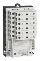
Electrically held lighting contactor, (convertible to mech. held), Amp rating 30A (tungsten 20A), 2 N.C. / 10 N.O. poles, 24V 60Hz / 20V 50Hz coil, Noncombination type, Enclosure NEMA type (open), No enclosure
