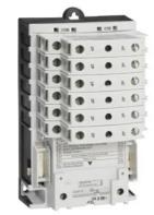
Electrically held lighting contactor, (convertible to mech. held), Amp rating 30A (tungsten 20A), 1 N.C. / 7 N.O. poles, 575-600V 60Hz/550V 50Hz coil, Non-combination type, Enclosure NEMA type (open), No enclosure
