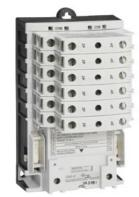
Electrically held lighting contactor, (convertible to mech. held), Amp rating 30A (tungsten 20A), 1 N.C. / 5 N.O. poles, 347V 60Hz coil, Non-combination type, Enclosure NEMA type (open), No enclosure
