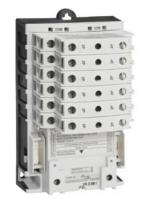
Electrically held lighting contactor, (convertible to mech. held), Amp rating 30A (tungsten 20A), 0 N.C. / 3 N.O. poles, 24V 60Hz / 20V 50Hz coil, Non-combination type, Enclosure NEMA type (open), No enclosure
