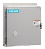
Mechanically held lighting contactor, Contactor amp rating 60Amp 0NC \_ 2NO poles, 110VAC 50HZ/120VAC 60HZ coil, Non-combination type, Encl NEMA type 4X 304 S-steel Water/dust tight noncorrosive
