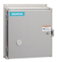
Mechanically held lighting contactor, Contactor amp rating 30A, 0 N.C. / 2 N.O. poles, 110VAC 50HZ/120VAC 60HZ coil, Non-combination type, Encl NEMA type 4X 304 S-Steel, Water/dust tight noncorrosive
