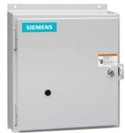
Mechanically held lighting contactor, Contactor amp rating 100A, 0 N.C. / 4 N.O. poles, 110VAC 50HZ/120VAC 60HZ coil, Non-combination type, Enclosure NEMA type 12, Dust/drip proof for indoors
