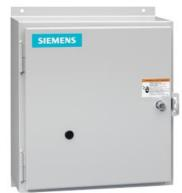
Mechanically held lighting contactor, Contactor amp rating 60Amp 0NC \_4NO poles, 277VAC 60HZ coil, Non-combination type, Enclosure NEMA type 12, Dust/drip proof for indoors
