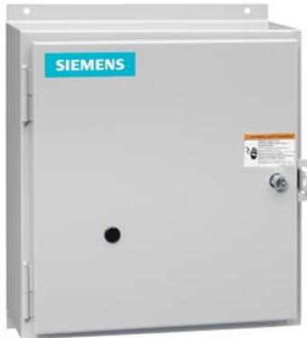
Mechanically held lighting contactor, Contactor amp rating 60A, 0 N.C. / 4 N.O. poles, 110VAC 50HZ/120VAC 60HZ coil, Non-combination type, Enclosure NEMA type 12, Dust/drip proof for indoors
