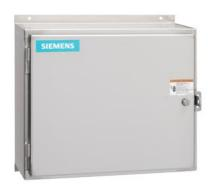
Mechanically held lighting contactor, Contactor amp rating 30A, 0 N.C. / 8 N.O. poles, 277VAC 60HZ coil, Non-combination type, Enclosure NEMA type 12, Dust/drip proof for indoors
