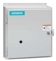
Mechanically held lighting contactor, Contactor amp rating 30A, 0 N.C. / 3 N.O. poles, 277VAC 60HZ coil, Non-combination type, Enclosure NEMA type 12, Dust/drip proof for indoors
