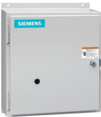
Mechanically held lighting contactor, Contactor amp rating 30Amp 0NC \_ 3NO poles, 220VAC 50HZ / 240VAC 60HZ coil Non-combination type, Enclosure NEMA type 12, Dust/drip proof for indoors
