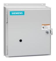
Mechanically held lighting contactor, Contactor amp rating 30Amp 0NC  $\_$  3NO poles, 24VAC 60HZ coil, Non-combination type, Enclosure NEMA type 12, Dust/drip proof for indoors
