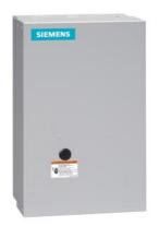
Mechanically held lighting contactor, Contactor amp rating 100A, 0 N.C. / 5 N.O. poles, 110VAC 50HZ/120VAC 60HZ coil, Non-combination type, Enclosure NEMA type 1, Indoor general purpose use
