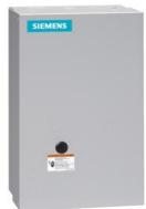
Mechanically held lighting contactor, Contactor amp rating 100A, 0 N.C. / 4 N.O. poles, 277VAC 60HZ coil, Non-combination type, Enclosure NEMA type 1, Indoor general purpose use
