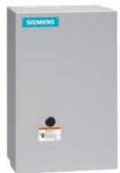
Mechanically held lighting contactor, Contactor amp rating 100A, 0 N.C. / 3 N.O. poles, 277VAC 60HZ coil, Non-combination type, Enclosure NEMA type 1, Indoor general purpose use
