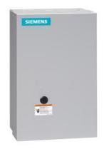
Mechanically held lighting contactor, Contactor amp rating 100A, 0 N.C. / 3 N.O. poles, 220VAC 50HZ/240VAC 60HZ coil, Non-combination type, Enclosure NEMA type 1, Indoor general purpose use
