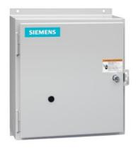
Mechanically held lighting contactor, Contactor amp rating 30A, 0 N.C. / 8 N.O. poles, 550VAC 50HZ/600VAC 60HZ coil, Non-combination type, Enclosure NEMA type 1, Indoor general purpose use
