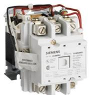
Mechanically held lighting contactor, Contactor amp rating 60A, 0 N.C. / 5 N.O. poles, 550VAC 50HZ/600VAC 60HZ coil, Non-combination type, Enclosure NEMA type (open), No enclosure
