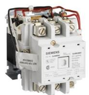
Mechanically held lighting contactor, Contactor amp rating 60A, 0 N.C. / 3 N.O. poles, 277VAC 60HZ coil, Non-combination type, Enclosure NEMA type (open), No enclosure
