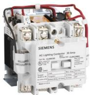
Mechanically held lighting contactor, Contactor amp rating 30A, 0 N.C. / 4 N.O. poles, 277VAC 60HZ coil, Non-combination type, Enclosure NEMA type (open), No enclosure
