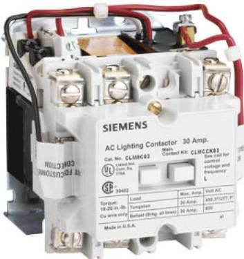
Mechanically held lighting contactor, Contactor amp rating 30A, 0 N.C. / 4 N.O. poles, 208VAC 60HZ coil, Non-combination type, Enclosure NEMA type (open), No enclosure
