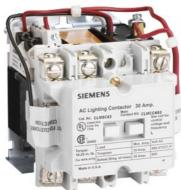
Mechanically held lighting contactor, Contactor amp rating 30A, 0 N.C. / 3 N.O. poles, 24VAC 60HZ coil, Non-combination type, Enclosure NEMA type (open), No enclosure
